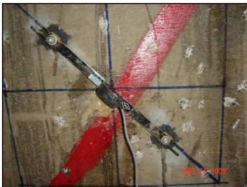
Fig.18 Linear Potentiometer's, Accelerometers and Strain Transducers in place for testing under the bridge
