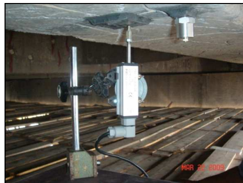
Fig.18 Linear Potentiometer's, Accelerometers and Strain Transducers in place for testing under the bridge
